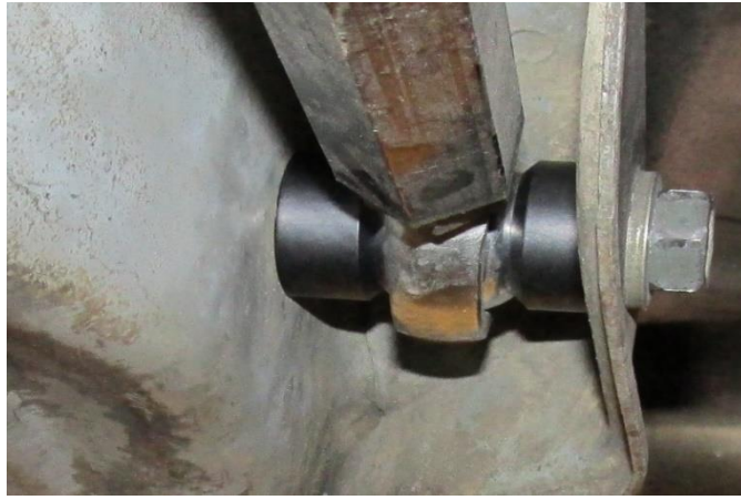
Figure 4: Rear Tie Rod Installation
