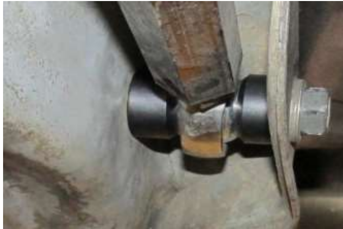
Rear Tie Rod Installation
