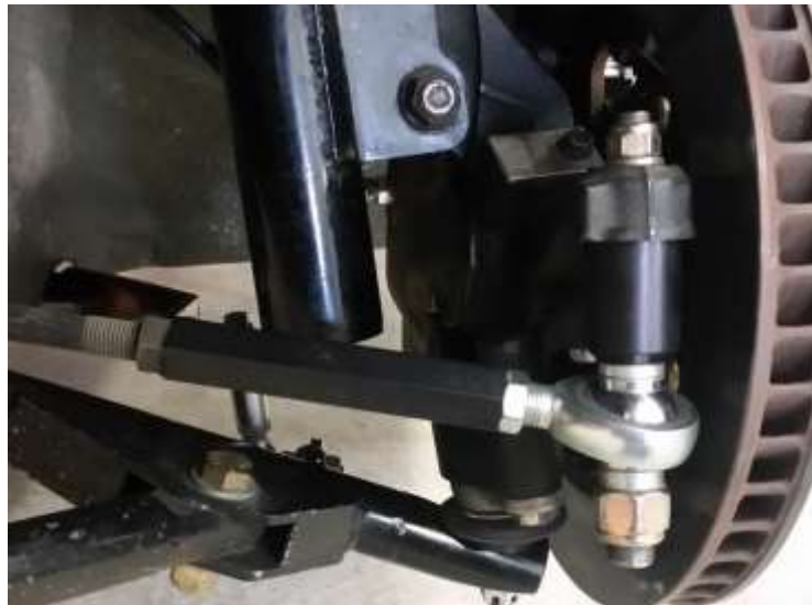
Front Tie Rod Installation
