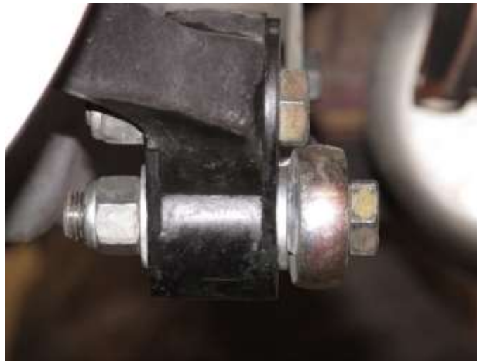
Rear Tie Rod Installation
